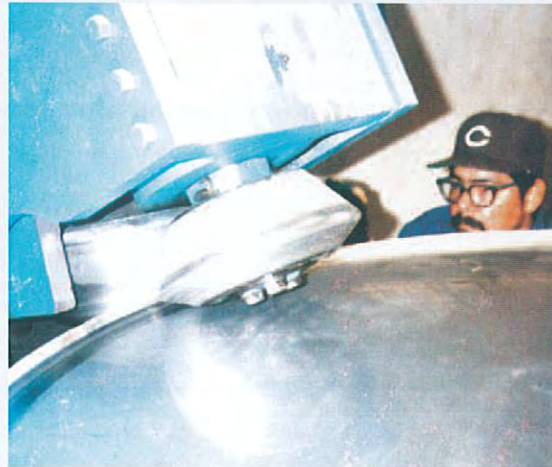
Bottoms and tops have full radius rolled corners for reduced weld distortion and ease of cleaning.
