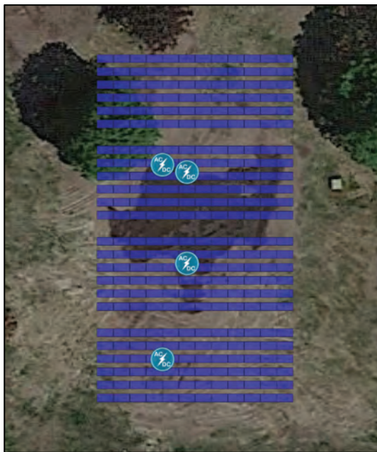
Figure 10: 99.4 kW Solar PV Array Designed for Net Metering
