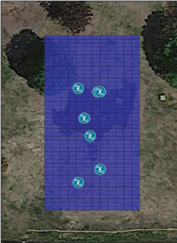
Figure 12: 186.3 kW Rooftop Solar PV Array for Net Zero Energy
