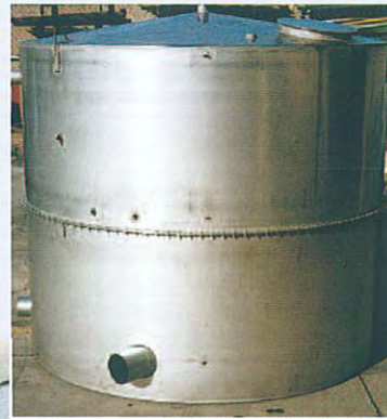
Bottoms and tops have full radius rolled corners for reduced weld distortion and ease of cleaning.
