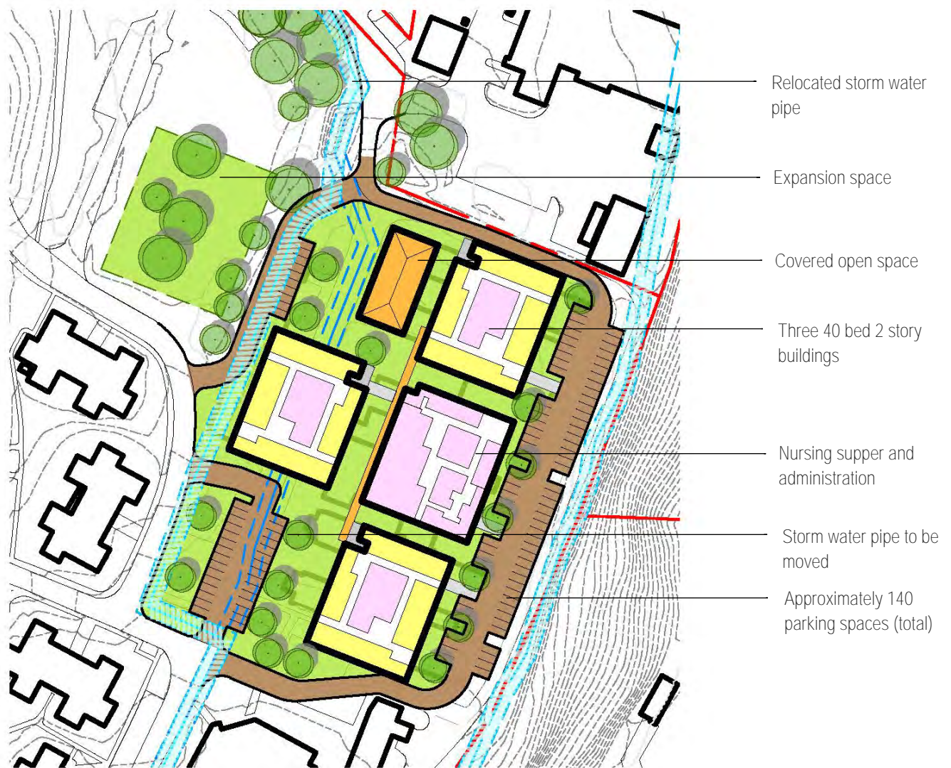
Figure 28 Conceptual site plan of a 2-story nursing facility on the Northwest Corner (Area 1)
